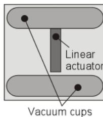
**Figure 12 - Two vacuum cups (1 actuated, 1 fixed) and vertical movement (on the left)**
