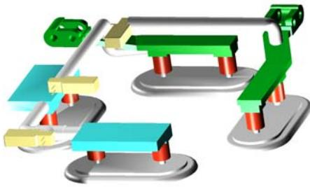
**Figure 5 - The cups and vacuum ducts**
