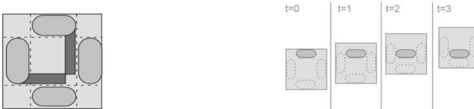
**Figure 14 - Four vacuum cups (the left and the bottom are fixed) and vertical path**
