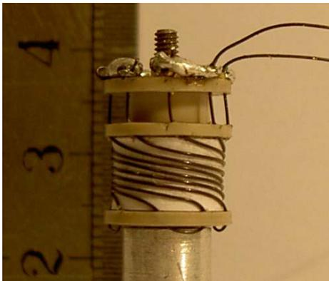
Figure 13. Spiral SMA gripper.
