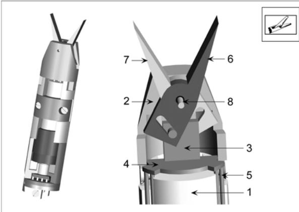
**Figure 10.** Gripper with wrist.
