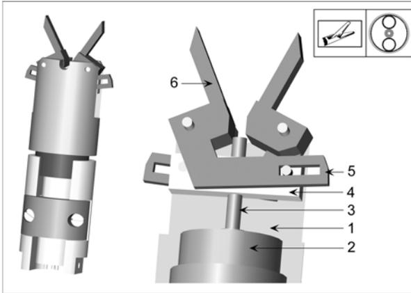
**Figure 3.** Motorised gripper.
