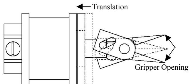
**Figure 5.** Gripper opening-closure principle
