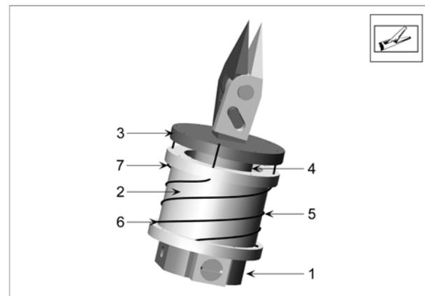
**Figure 12.** Spiral SMA gripper.
