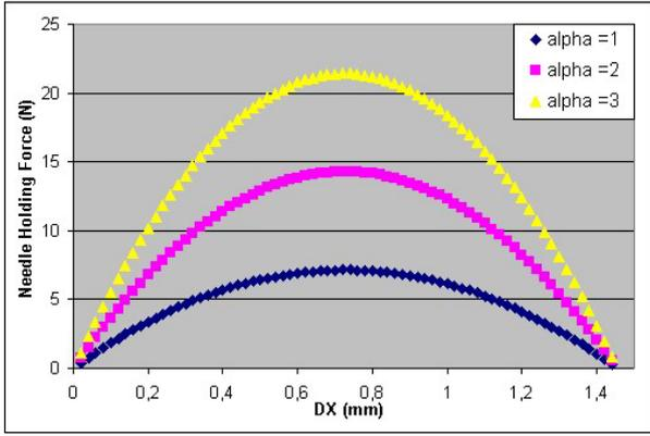
**Figure 7.** Needle holding force vs Displacement.
