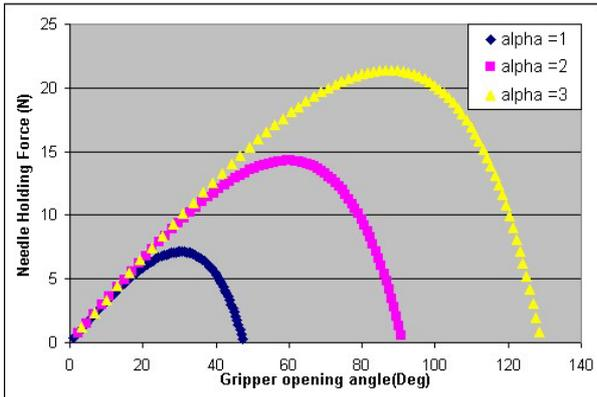
**Figure 8.** Needle holding force Opening angle.
