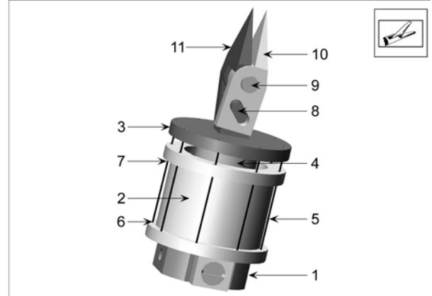
**Figure 9.** Parallel SMA gripper.
