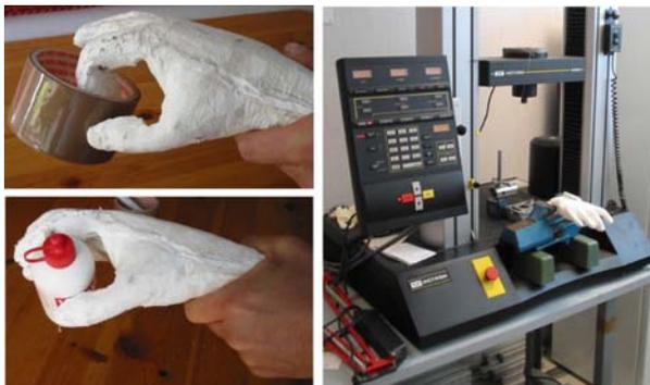
**Figure 3.** Hand grasping and tests on the prototype
